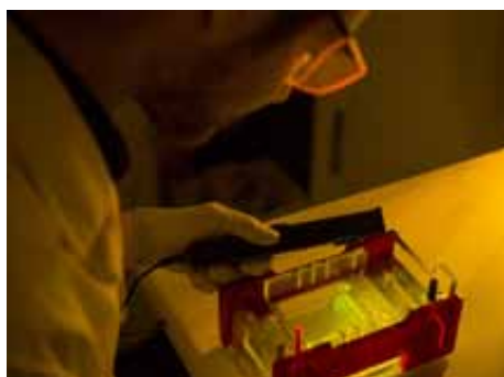
Fig. 1: The FastGene® Blue/Green LED Flashlight is very handy. The Blue/Green LEDs can be used to excite gels stained with red or green dyes, such as Midori Green Direct shown here.
