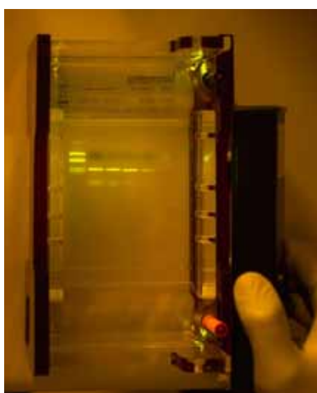
Fig. 2: You can detect fluorescent nucleic acid dyes in any clear electrophoresis unit.
